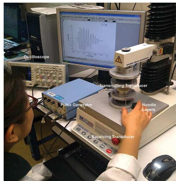
Fig. 1. Ultrasonic setup used to evaluate noodle dough sheets.
